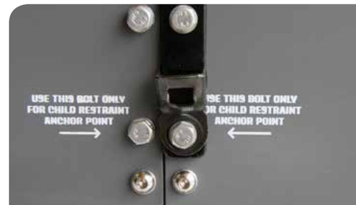
The same **second bolt down** from the top only can be used as a Cargo Barrier mount and a Child Restraint point from the same bolt if needed. (see image above)
